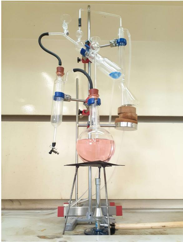
Figure 1. Semi-micro Kjeldahl distillation
