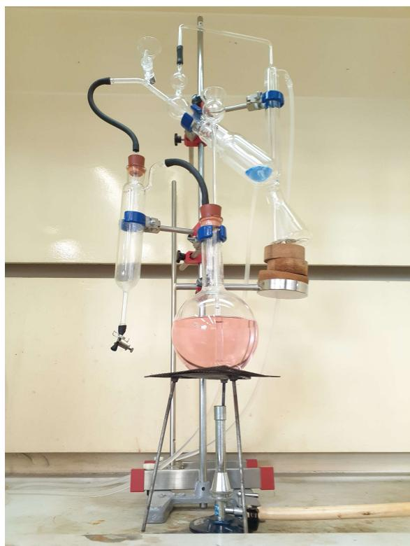
Figure 1. Semi-micro Kjeldahl distillation
